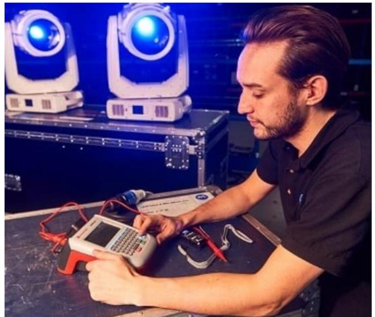
PAT testing is the examination of electrical appliances and equipment to see if maintenance is required and ensure they are safe for continued use. Many electrical safety defects can be found by visual examination, but some types of defect can only be found by carrying out testing.
